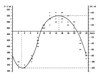
Fig. 2: Measurement of  $2\delta I$ . The points give the measurements at the even hours for the days from the 9th to the 13th February 1984.
