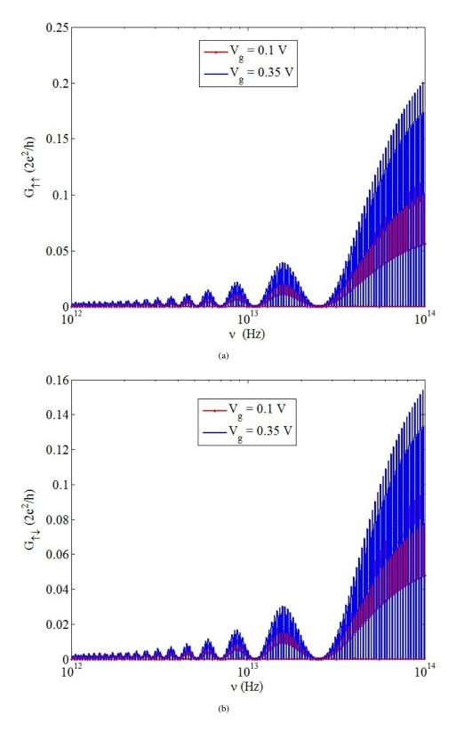
Fig. 1: The variation of conductance with frequency at two different gate voltages for (a) parallel spin alignment and (b) antiparallel spin alignment.
