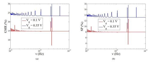
Fig. 2: The variation of (a) GMR and (b) SP with frequency at two different gate voltages.
