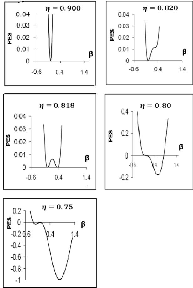
Fig. 1: Potential energy surface (PES) equation (3) for  $N=10$  calculated with IBM without normalization along the axial trajectory  $\gamma = 0^\circ, 60^\circ$  as a function of the shape parameter  $\beta$ . The curves describe the first order shape phase transition between spherical to prolate deformed U(5)-SU(3) for control parameter  $\eta$ :  $\eta = 0.900$ ,  $\eta = 0.820$  (spinodal),  $\eta = 0.818$  (critical point),  $\eta = 0.800$  (antispinodal) and  $\eta = 0.750$ .
